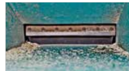
Cutting system/drum - two reversible blades ensure a clean, retracting cut. Blunt blades can be rotated.
